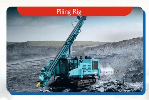
A construction machine mainly used to drill/create piles in soil, clay, etc.
